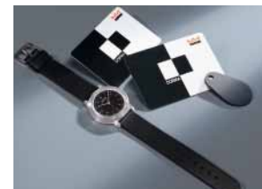
Access cards, transponder keys and wristwatches by Junghans with integrated transponder chip
