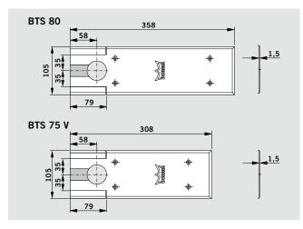
Calculating the necessary length of spindle extension: Extension = X – Floor clearance (normally 8 mm) Collar height Z of the extended spindle inserts = Spindle extension length + 3 mm (collar height of the standard spindle insert)
